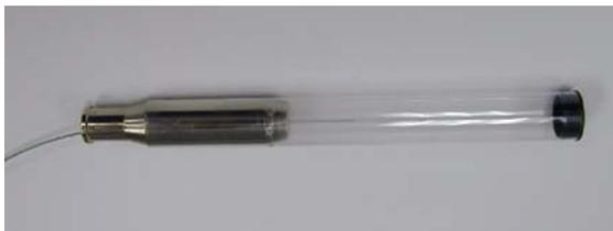
**Figure 33** Protective sleeve on needle assembly.
