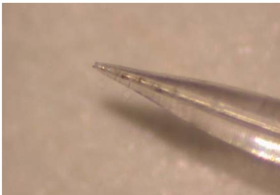
**Figure 21** Needle tip clogged with metal flakes, or fragments of conductive ferrule, as well as glass fragments.
