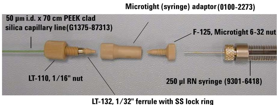
**Figure 26** Components of syringe infusion assembly
