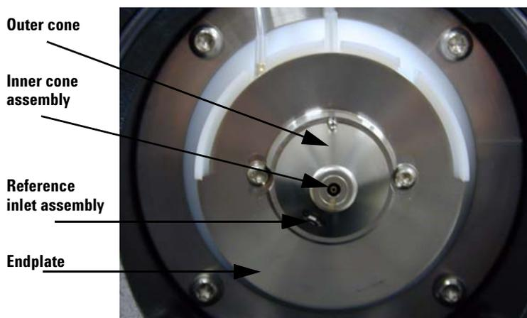
**Figure 43** DNS installed
