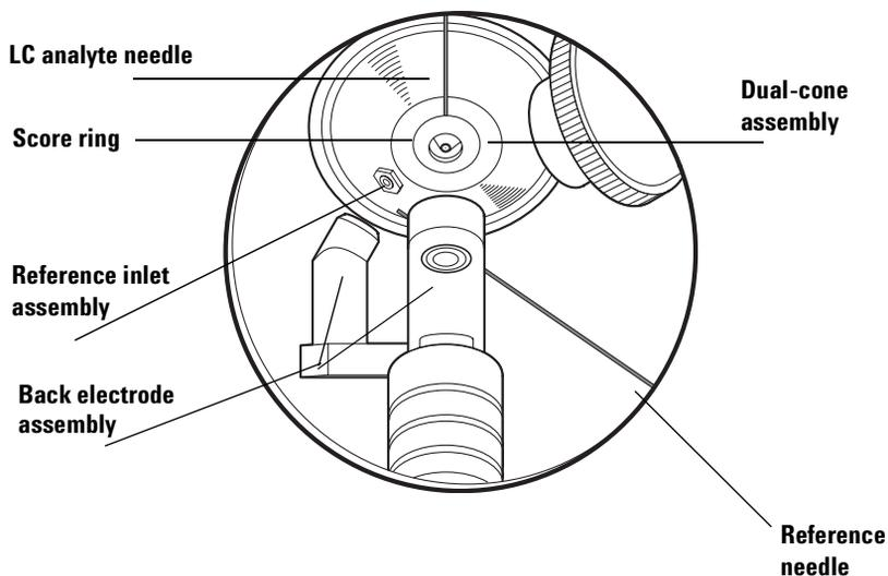
**Figure 44** DNS assemblies and needle positions
