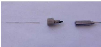
**Figure 24** Needle, needle nut, ferrule and union.
