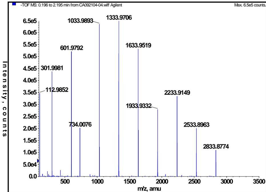
Figure 9 Sample negative ion mass spectrum of ES-TOF Tuning Mix.
