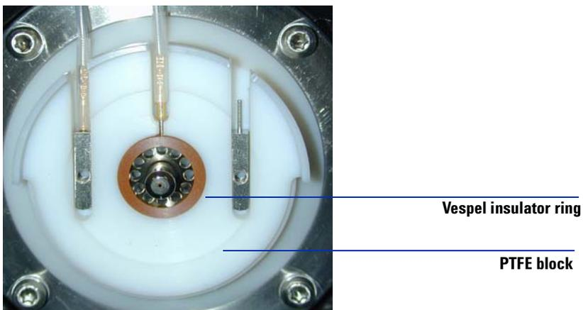
**Figure 42** Spray shield, capillary cap, and endplate removed.
