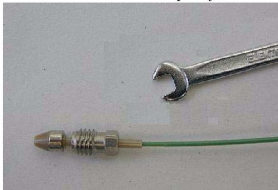
**Figure 27** Capillary transfer-line and 4 mm wrench
