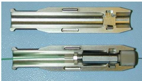
**Figure 31** The needle/union/transfer assembly seated into the union holder.
