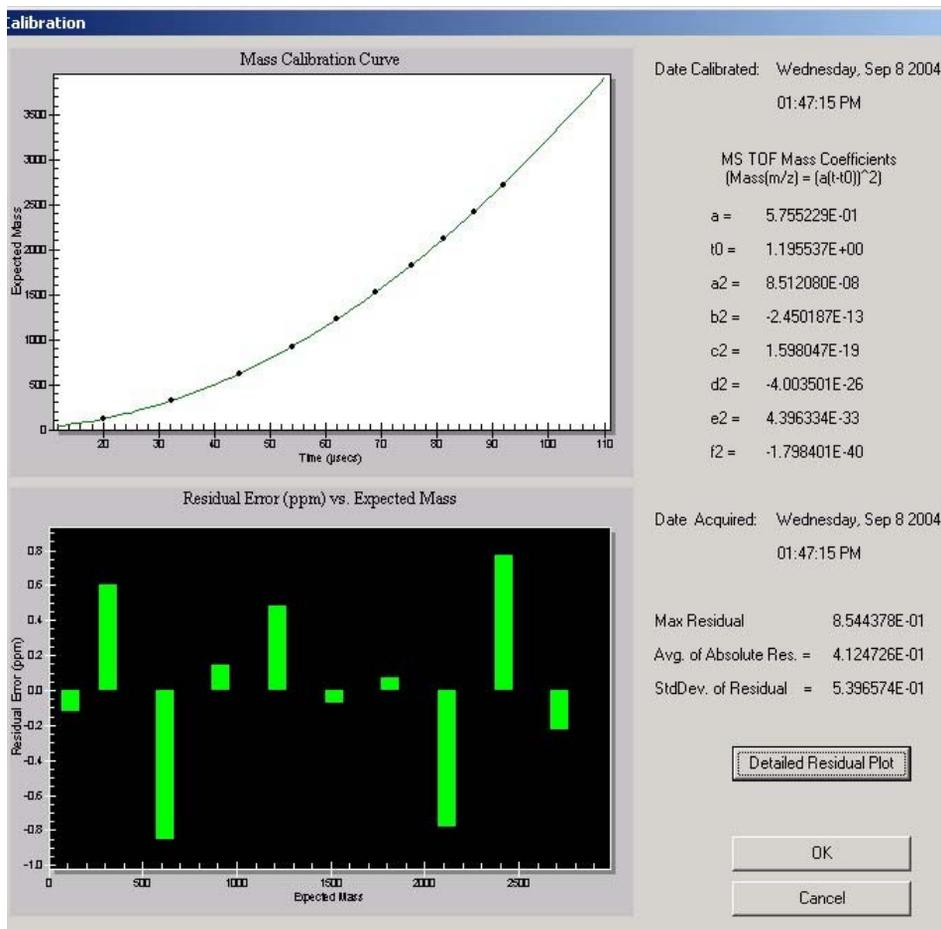
**Figure 7** Calibration results (positive ion mode)
