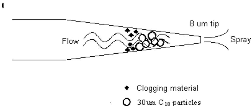
**Figure 37** How C18 particles help prevent clogging
