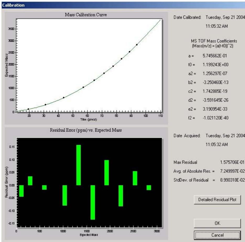
**Figure 10** Calibration results (negative ion mode)
