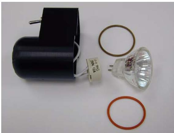
**Figure 20** Lamp detached from receptacle
