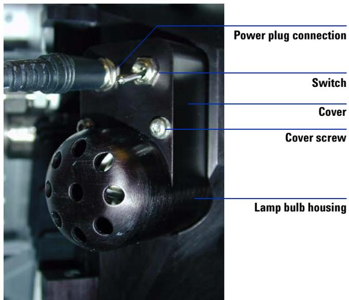
**Figure 35** Lamp, switch, cover and cover screw
