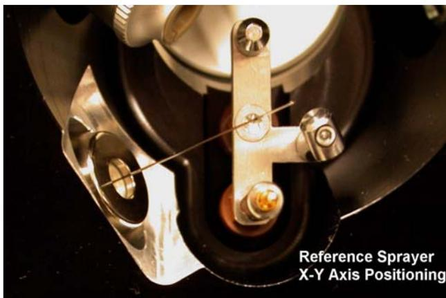
**Figure 18** Reference sprayer X-Y axis positioning
