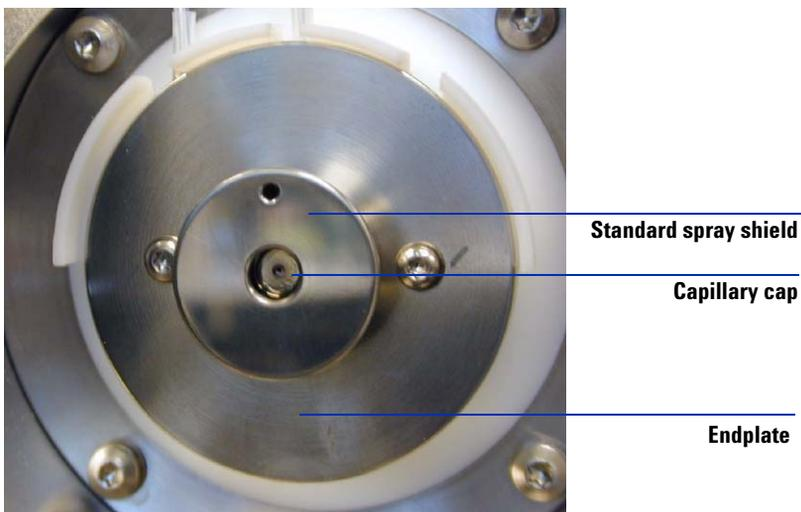
**Figure 41** Standard spray shield and capillary cap for ESI or APCI
