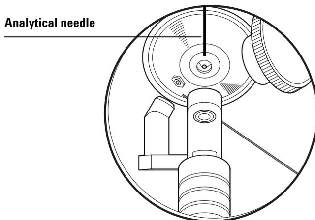
**Figure 3** Alignment of PicoTip for tuning or calibration
