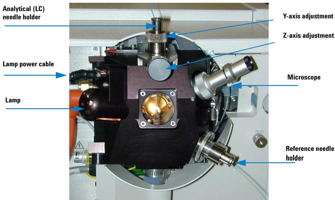
**Figure 1** Dual nanospray ion source.
