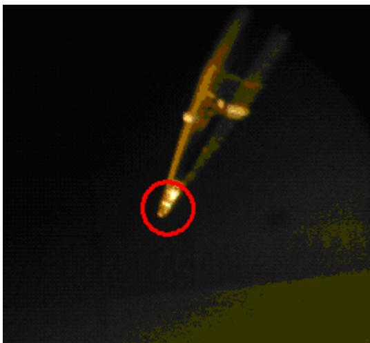
**Figure 39** 30  $\mu\text{m}$  C18 particles aggregated just upstream of the needle tip opening. This photo actually shows too much C18 material, which is the result of dipping the needle into the suspension for 5 seconds. Only a barely discernible amount is needed to prevent clogging.
