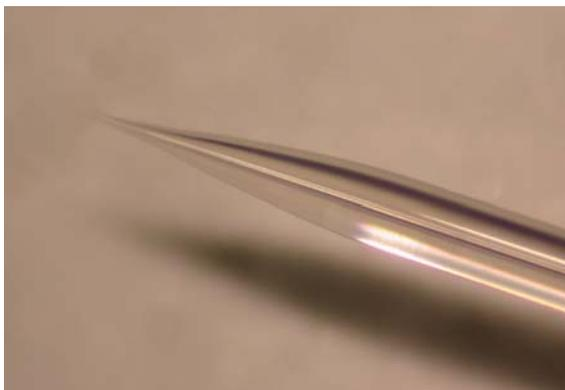
**Figure 22** Clean needle tip
