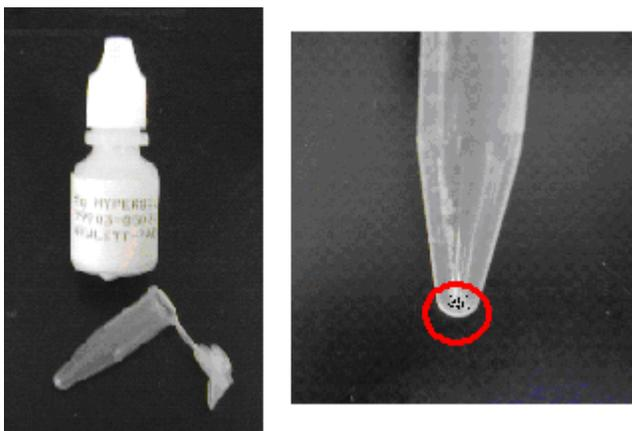
**Figure 38** C18 beads barely visible at bottom of vial.
