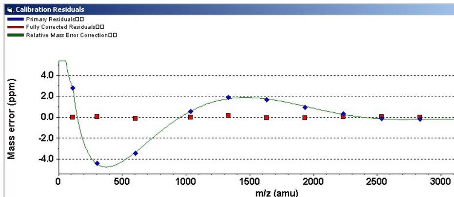
**Figure 11** Detailed residual plot from negative ion calibration
