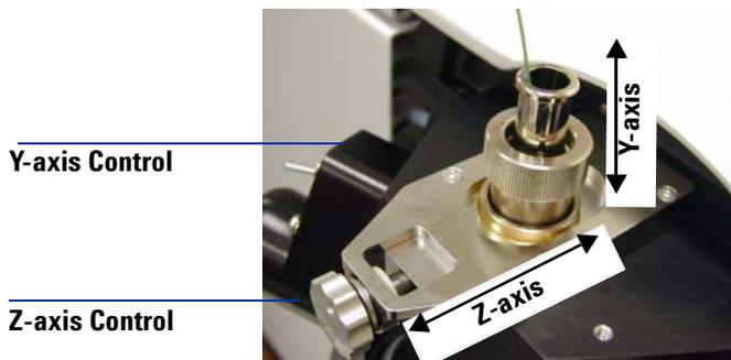
**Figure 12** Adjustment of the needle position in the vertical direction uses the Y-axis control knob. Adjustment of the horizontal direction, between the back electrode and inlet capillary, uses the Z-axis control knob.
